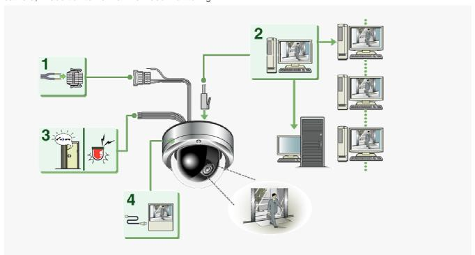
1 Connect the power cable to the power terminals.
